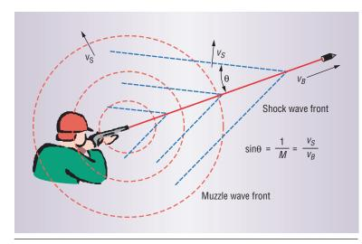
Figure 1. Acoustic events generated by a shot. The muzzle blast produces a spherical wave front that travels at the speed of sound  $(v_s)$  from the muzzle. The supersonic projectile generates a shock wave in every point of the trajectory, producing a cone-shaped wave front (assuming the speed of the projectile is constant  $v_{\rm B}$ ). The projectile's Mach number M determines the angle of the shockwave cone.
